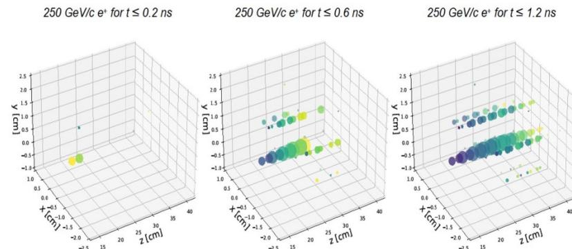
Timing development of an electromagnetic shower in HGCAL prototype
